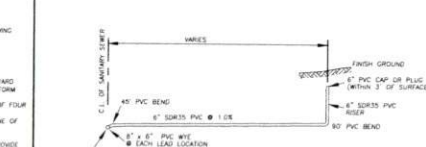
SANITARY SEWER LEAD
