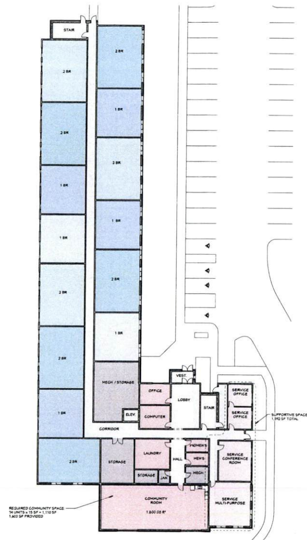
FIRST FLOOR PLAN 1/16" = 1'-0"
