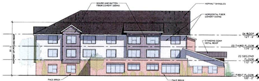
SOUTH ELEVATION 392' x 1'-0"
