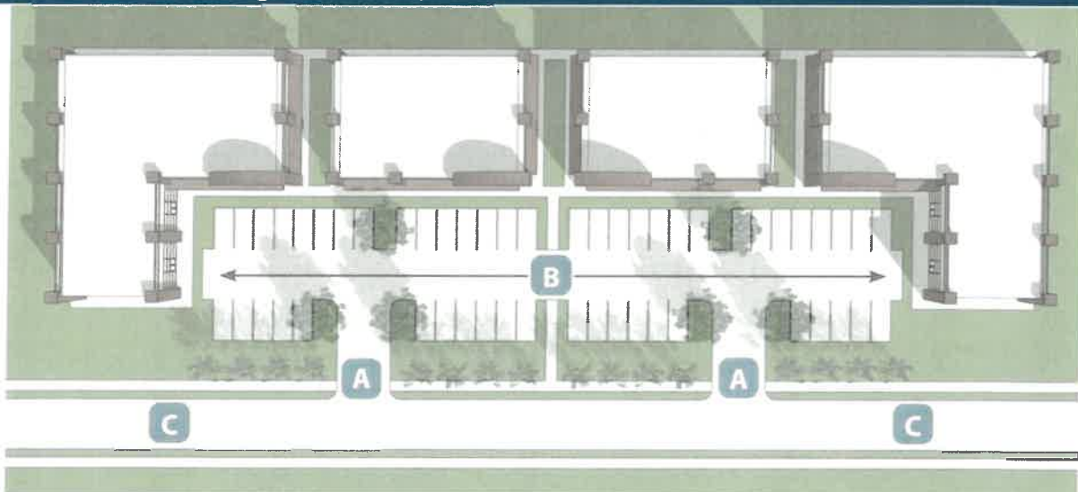
Figure Notes: OTES: A = Shared Access B = Cross Access C = Primary Street
